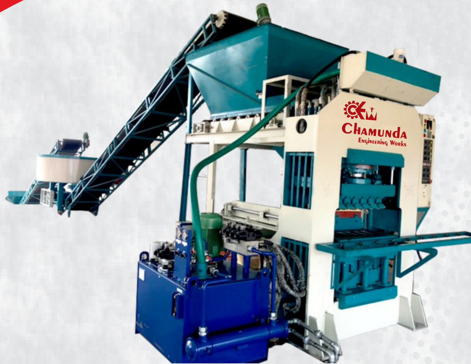
► Automatic Flyash Bricks Making Machine Capacity - Heavy Hydraulic 4 Bricks Press Pallet Size - 480 X 300 X 15 mm Batch Size - 400 to 500 kg. Production Capacity : 1400 to 1600 Bricks / Hour No. of Bricks / Stroke : 4 Bricks / Stroke
